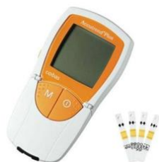
Figure 1. Accutrend Plus Lactic Acid Meter, Roche Brand
